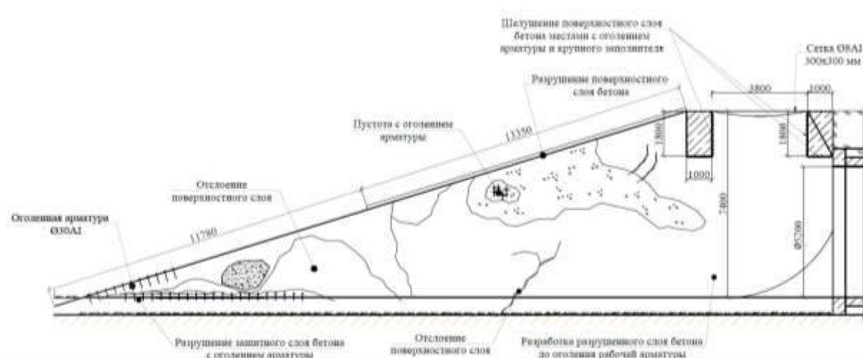
Figure 3 – The current state of the southern portal (left wall)
